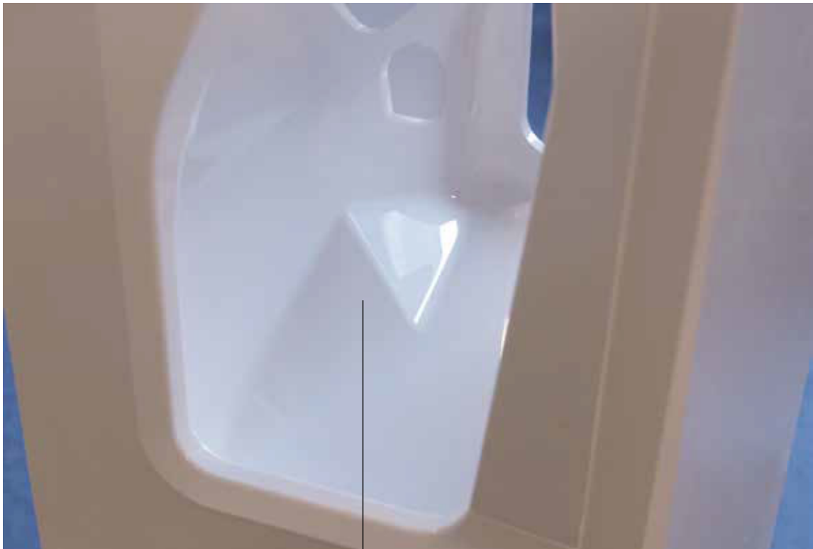
Triangular flow deflector reduces noise
